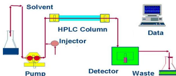
Fig-1: Flow Diagram of HPLC
